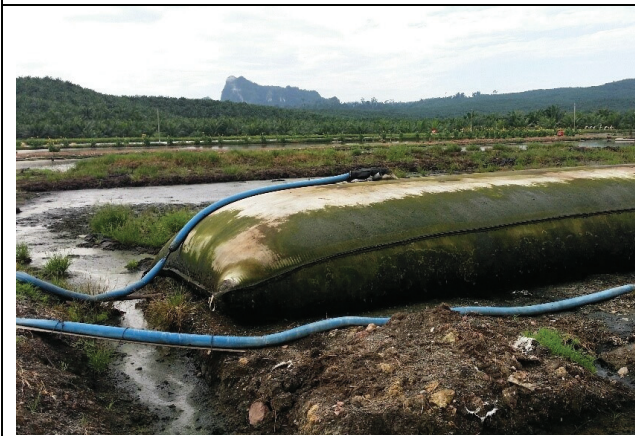
Geotube at Baturong POM.
